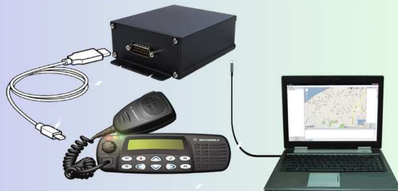
Base Station Unit(BSU)
